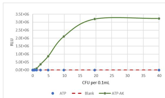
**Figure III - A: Comparison of the AK method (solid line) and the ATP method (blue circles). CFU-RLU dependence for Propionibacterium acnes. (A. - general dependence; The horizontal dashed line is a 3 times blank baseline)**
