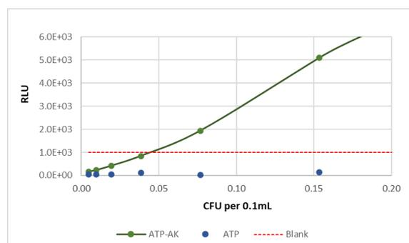
**Figure III - B: Comparison of the AK method (solid line) and the ATP method (blue circles). CFU-RLU dependence for Propionibacterium acnes. (B. - dependence at low concentrations of the microorganism. The horizontal dashed line is a 3 times blank baseline)**
