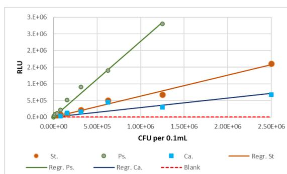
**Figure IV A, CFU-RLU dependence ATP method. Pallchek™ Rapid Microbiology System. (B - dependence at low concentrations of the microorganisms. The horizontal dashed line is a 3 times blank baseline)**
