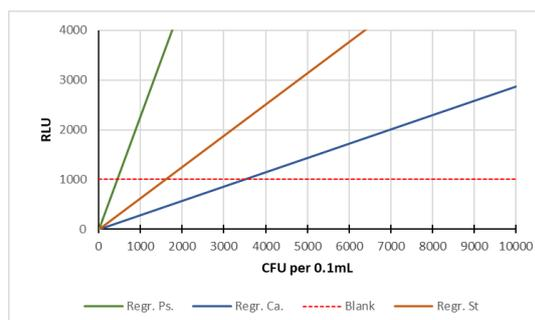
**Figure IV - B: CFU-RLU dependence ATP method. Pallchek™ Rapid Microbiology System. (B. - dependence at low concentrations of the microorganisms. The horizontal dashed line is a 3 times blank baseline)**
