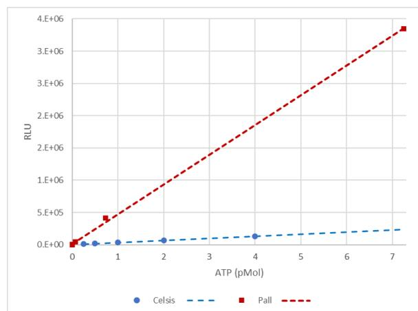
Figure - I: Calibration curves for two luminometers: Celsis and Pall.
