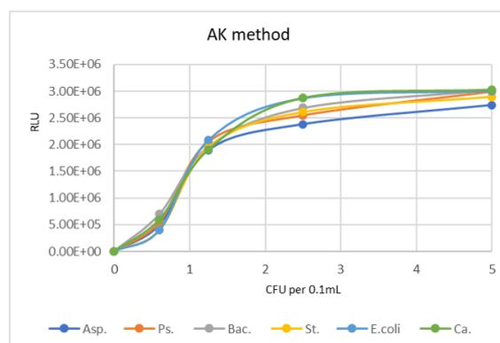
Figure II - B: Dependence of the test result on the reference concentration of microorganisms in the sample in CFU units. (B. AK method)
