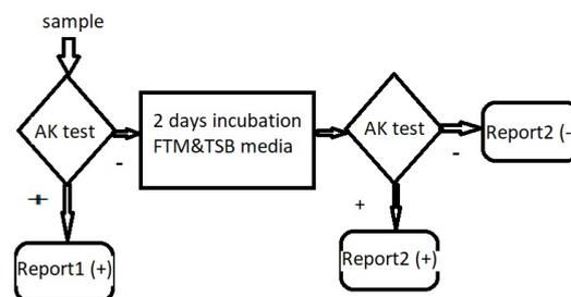
**Figure - VI. The scheme for the quantitative analysis of samples for sterility.**
